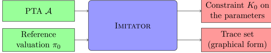
Figure 2: IMITATOR inputs and outputs in inverse method mode
