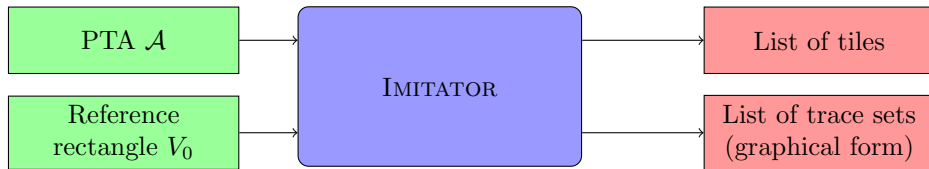
Figure 3: IMITATOR inputs and outputs in behavioral cartography mode
