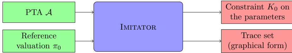
Figure 2: IMITATOR inputs and outputs in inverse method mode
